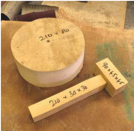
▲ Pic.1 The wood sizes: the bowl could be made bigger but the hammer size must be the same as over-enthusiastic cracking with too big a hammer could damage the bowl
